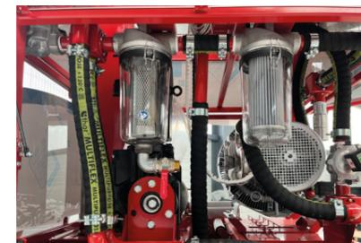
Filtering system for wet and dusty environments
