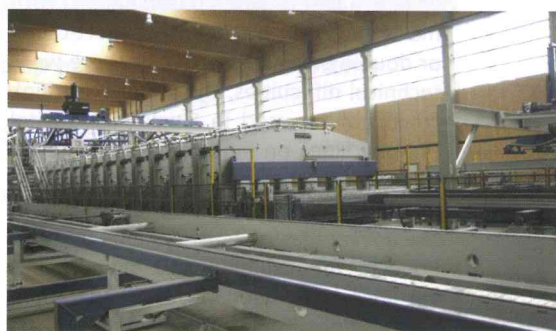
CLT press with modular belt conveyor and stacker in the background
